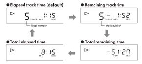
> Total remaining time and total elapsed time will not be displayed when program mode and/or repeat mode are active.
