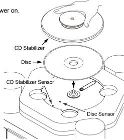
matically to read out the disc information. Approximately 5 seconds later the display will change to indicate the total number tracks and the total playing time.
