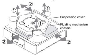
When packing the TL0 3.0 again for transportation insert the ① three smaller pads between the suspension covers and the floating chassis and the ② three bigger pads under the floating chassis.
