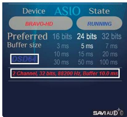
**Note:** Selecting ASIO Native at DSD Playback Method (refer to page 19), the bit rate and buffer size during DSD playback are fixed at 32 bits and 10.0 ms.
