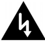
The lightning flash with arrowhead symbol, within an equilateral triangle, is intended to alert the user to potential shock hazards within the product's enclosure.
