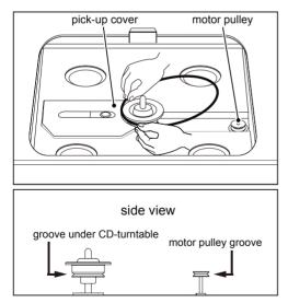
• Then mount the belt to the motor pulley groove. Using a pair of tweezers would be easier to mount.
