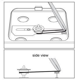
Be sure the belt is installed at the grooves and the belt is not twisted. Twist of the belt can be corrected easily by using a pair of tweezers moving the center shaft by hand.
