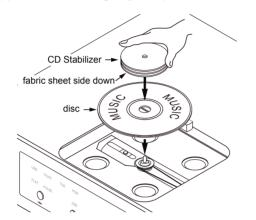
**Important**: Make sure that a disc and the CD stabilizer have been set correctly and laterally before closing the CD door.
