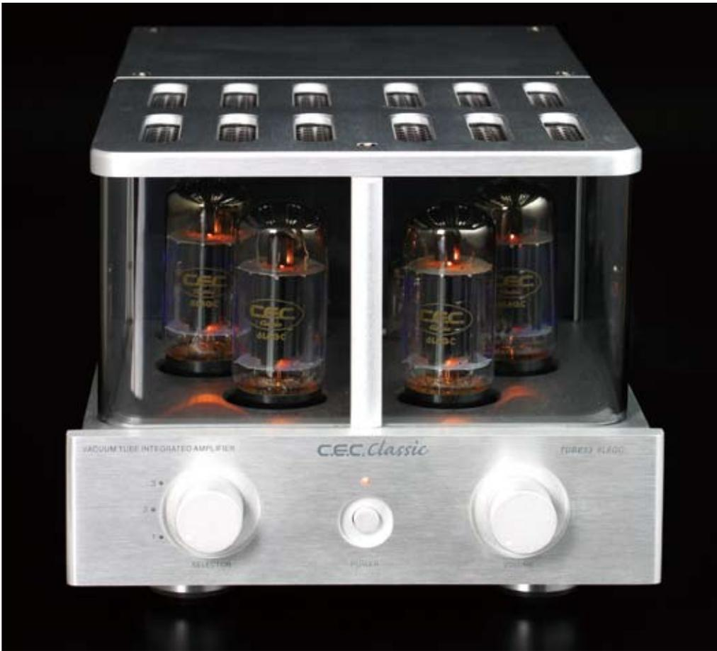
The TUBE53 is the CEC's first vacuum tube amplifier which achieves a 20W + 20W (8Ω) output. It offers high-power, high response and the ability to drive analogue signals with ease, even from digital media players.
